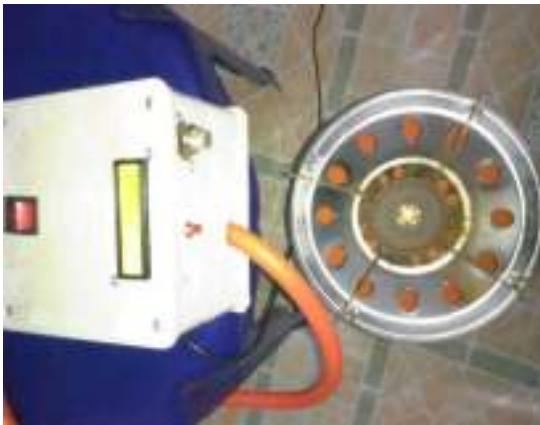
Fig.7(b): LPG detector higher than gas source Fig.7: LPG detector system testing set up
