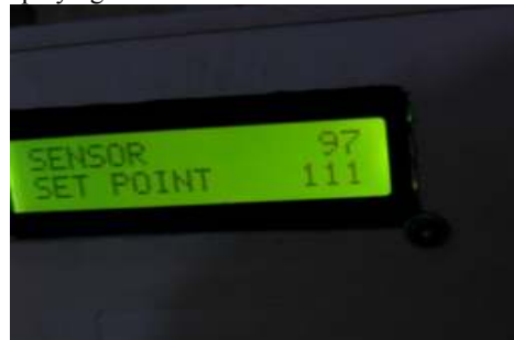
Fig.10: LPG detector system with gas concentration less than set reference.
