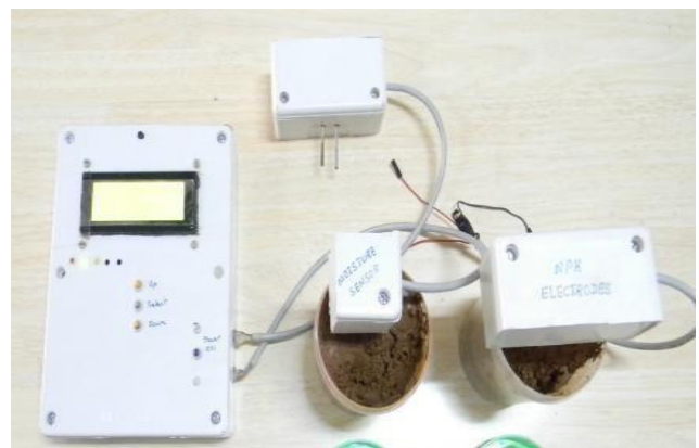
Figure 3: (a) Typical crystal display (b) an experimental setup of soil analyser
