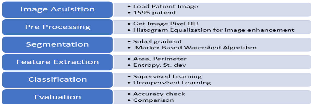
Figure 1 CT Image analysis steps for breast cancer detection
