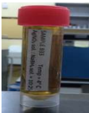
Sample B33: reaction temperature of 4°C Solution ratio of \text{AgNO}_3 : \text{NaBH}_4 of 10:25
