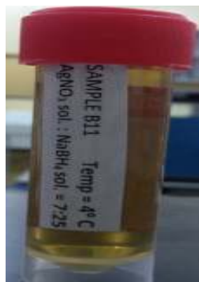
Sample B11: reaction temperature of 4°C Solution ratio of \text{AgNO}_3 : \text{NaBH}_4 of 7:25
