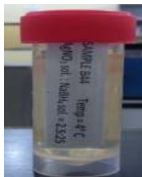
Sample B44: reaction temperature of 4°C Solution ratio of \text{AgNO}_3 : \text{NaBH}_4 of 2.5:25
