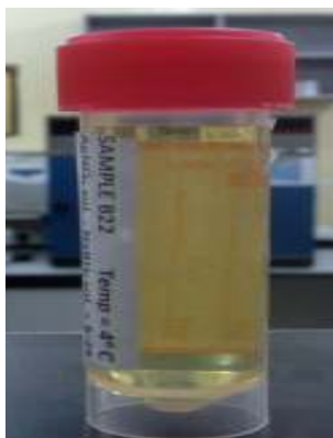
Sample B22: reaction temperature of 4°C Solution ratio of \text{AgNO}_3 : \text{NaBH}_4 of 5:25
