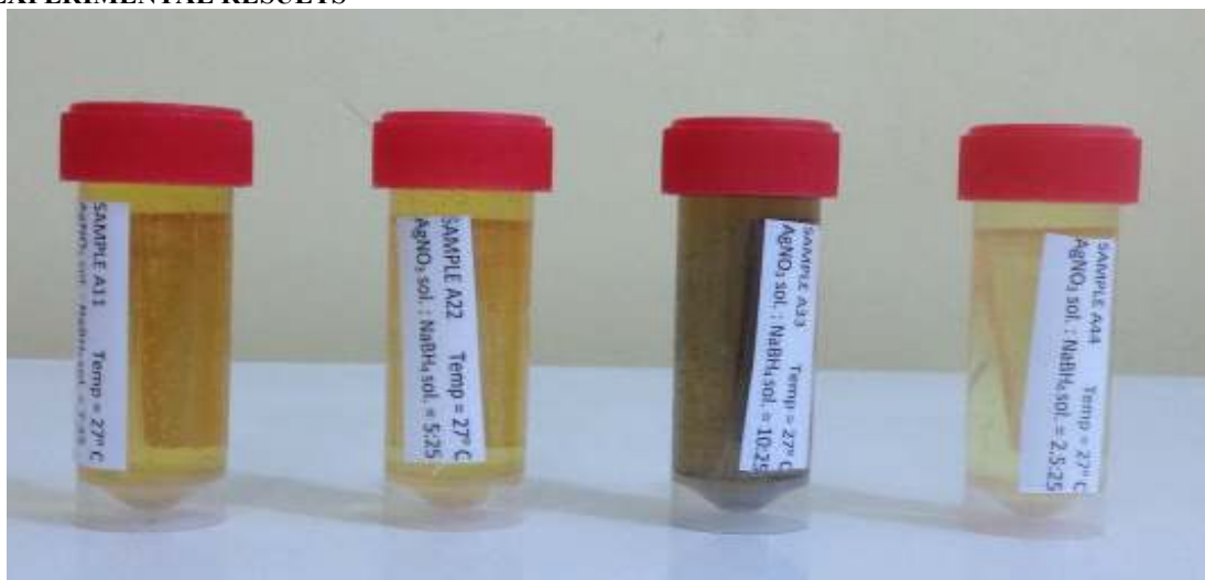
Figure 6 freshly prepared silver nanoparticles at room temperature using sodium borohydride as reducing agent and using different concentrations ratio
