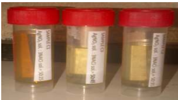
Sample C1 ( \text{AgNO}_3 sol : 3\text{NaCl} sol = 50:25), Sample C2 ( \text{AgNO}_3 sol : 3\text{NaCl} sol = 50:35), Sample C3 ( \text{AgNO}_3 sol : 3\text{NaCl} sol = 50:45)
