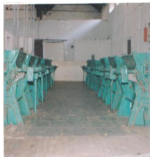
BATTERY OF DOUBLE ROLLER (DR) GINNING MACHINES
