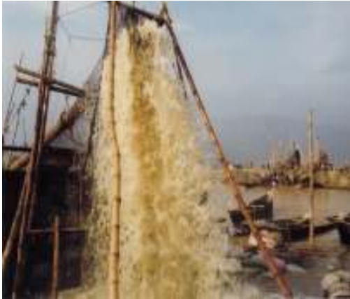
Boma machine through which stone withdrawn from 150-200feet deep of ground
